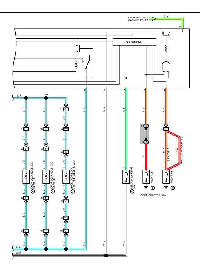
CURRENT ALWAYS FLOWS TO TERMINAL 8 OF THE DOOR LOCK CONTROL RELAY THROUGH POWER CB.
